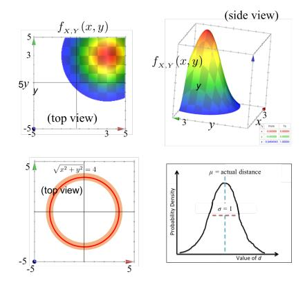
instrument reports that the object is 4 units away. Our instrument is not perfect: if the true distance was *t* units away, than the instrument will give a reading which is normally distributed with mean *t* and variance 1. Let's visualize the observation:
